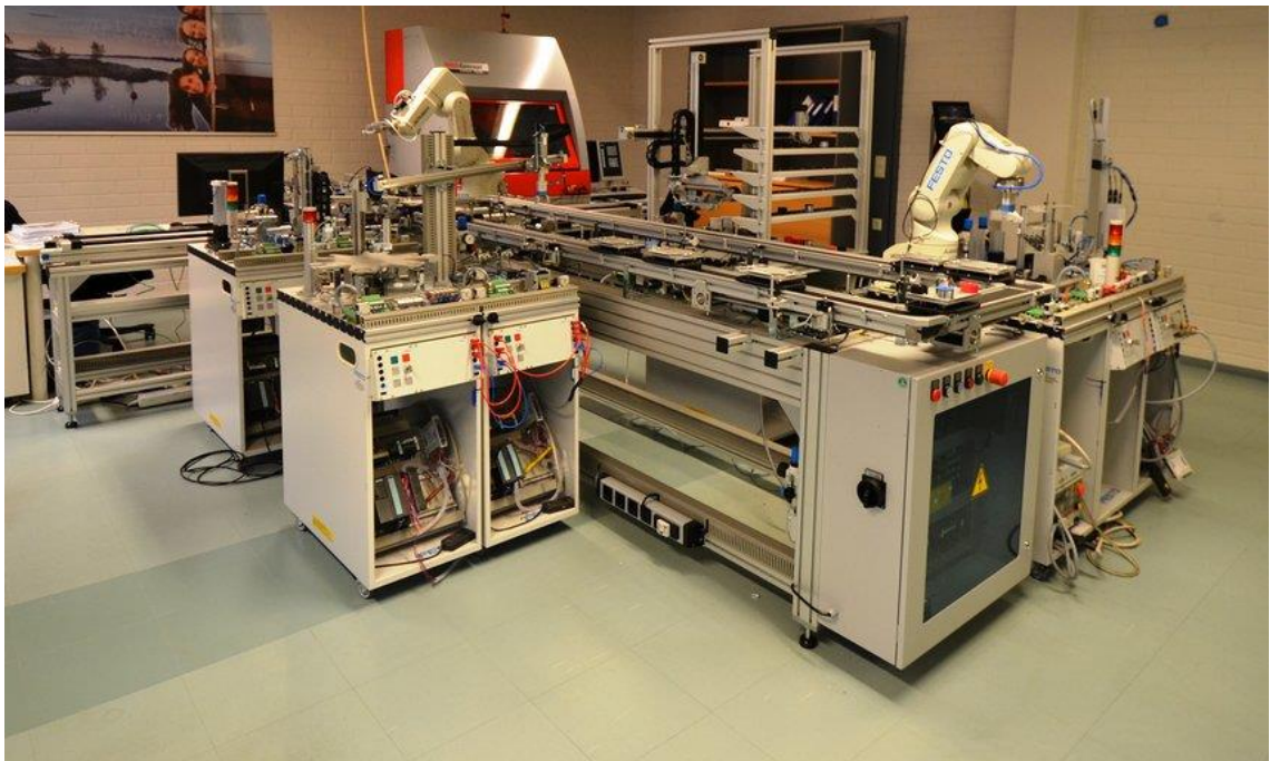
Figure 18: FESTO Multi-FMS on TUT FAST Laboratory facilities [61]
