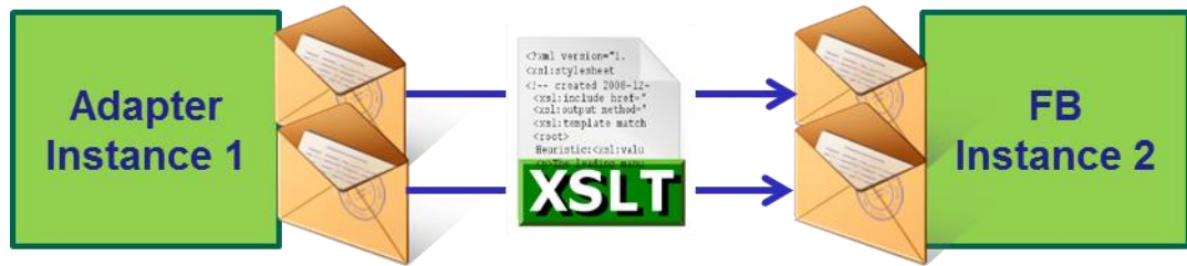
Figure 29: Connection of FBI thought XSL transformation of message types
