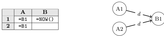
Fig. 5: Two cells depend on the same cell containing call to NOW() . If both cell A1 and A2 are evaluated in parallel and both recursively attempt to evaluate B1, their respective threads must agree upon which value B1 has evaluated to.
