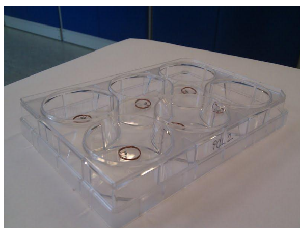
Figure 21: Handmade resonance sensors before biodegradable encapsulation
