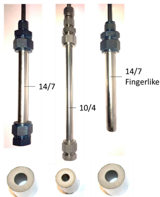
Figure 1. Sealed membranes with a cross-section; from left to right: A 14/7 mm outer/inner diameter (OD/ID) membrane, a 10/4 mm OD/ID membrane and a 14/7 mm OD/ID finger-like membrane.
