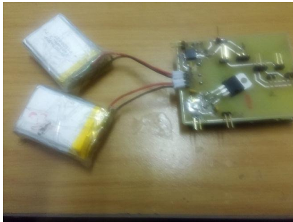
Figure 4-57: Battery connections to the EMG control board
