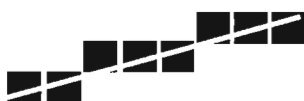
Figure 2-3: A line (in white) is rasterised into pixels (black squares). In moving from left to right, the value of y can only stay the same, or increment by one for each step.
