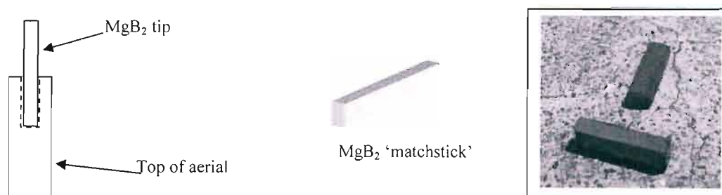
Figure 4-22: \text{MgB}_2 “matchstick” inserted into aerial tip, and matchstick pellets used.
