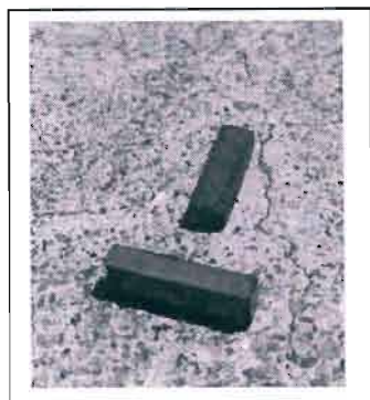
Figure 5-2: MgB 2 'matchstick' pellets. Each is 2x2x10 mm.
