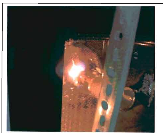
Figure 4-16: Small hydrogen plasma located at the aerial tip. This was a particularly hot, higher pressure plasma. At lower pressures, the colour is purple and the aerial does not glow such an intense bright orange/white.
