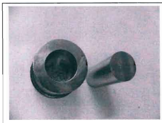
Figure 4-27: Die pieces used to press magnesium disc-shaped pellets.
