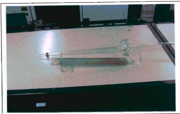
Figure 4-7: Two halves of the new chamber. The lower, thicker half is dark with a coating from an experiment.
