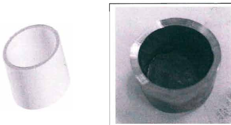
Figure 4-23: Another type of aerial tried. It was essentially nothing more than a 19 mm OD stainless steel tube (304 grade) sealed off at the bottom.
