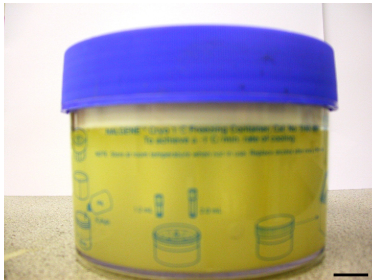
Figure 2.2: Freezing container, Mr Frosty, used for two-stage cooling.
