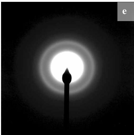
Figure 5.31 Amorphous silica in the clay fraction of sediments from Core 4 at 600 cm (a-c) and Core 3 at 450 cm (d). Typical diffuse diffraction rings produced by amorphous silica (e)
