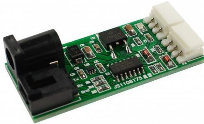
Figura 2.19 Dynamixel AX/MX bus Driver Board CDS55xx Fuente: http://robosavvy.com/store/dynamixel-ax-mx-bus-driver-board-cds55xx.html
