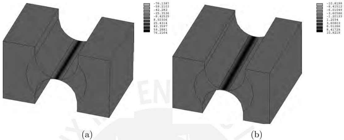
Figure 4.5: Bending stress \sigma_x in MPa: (a) ideal flexure hinge (b) non-ideal flexure hinge.
