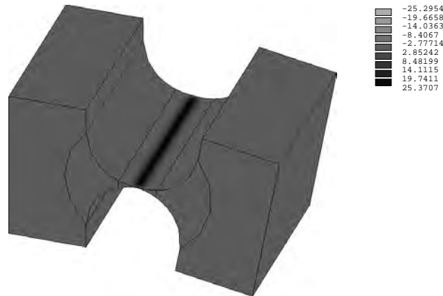
Figure 3.14: Out-of-plane stress \sigma_z in MPa for h = 0.05 mm.
