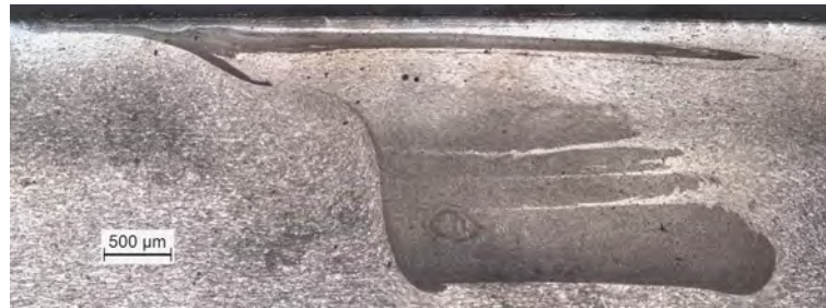
(b) T3 (1800 rpm; 40 mm/min)
