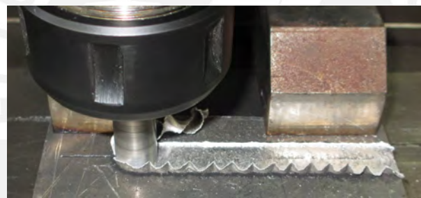
(a) Channel closing with a pinless tool
