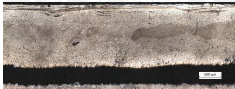
(a) F2 (1800 rpm; 20 mm/min)
