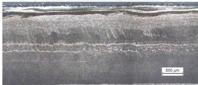
(a) T3 (2000 rpm; 20 mm/min)
