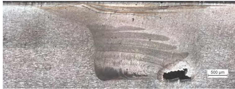
(a) S1 (1600 rpm; 20 mm/min)
