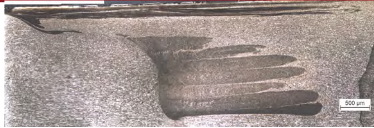
(a) T1 (1600 rpm; 20 mm/min)
