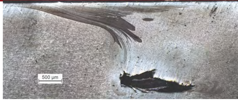
(a) F7 (1600 rpm; 60 mm/min)
