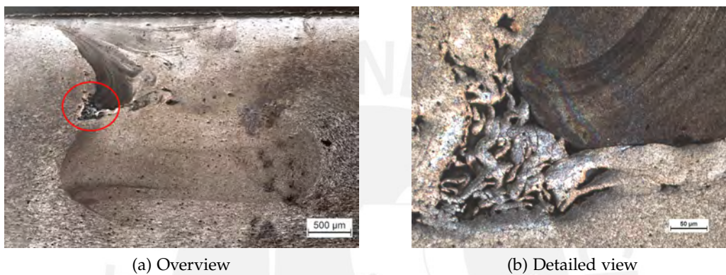
Figure 5.6: Sheared metal particles in the defect of sample C4 (1600 rpm; 40 mm/min)
