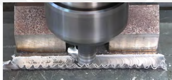
(b) FSP of the closed channel
