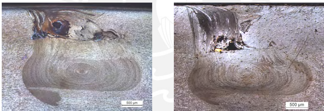
(a) C1 (1600 rpm; 20 mm/min)
