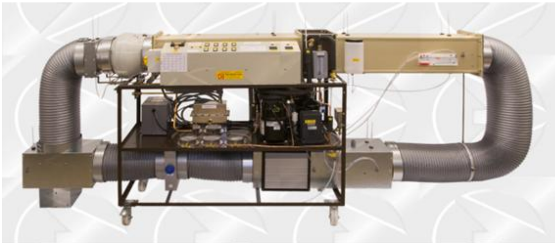
Figure 2 : Air treatment station A660 Base Unit with A661B Recirculation Duct Upgrade [8].
