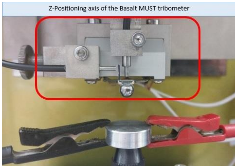
Figure 58: The Z-Positioning axis marked in red is moved during the “Z Positioning” event
