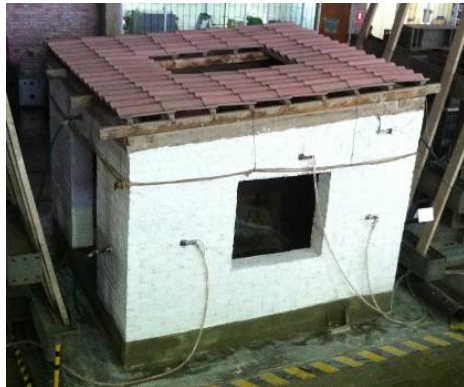
Model on the shaking table
