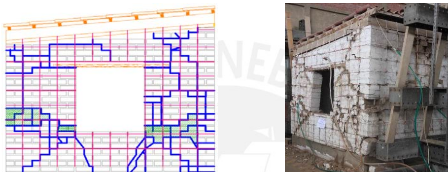
Figure 8. Sketch of damage pattern and general view of the model after all shaking phases.
