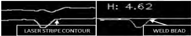
Fig. 7 Image after, threshold of 0.8 and morphological operations (a) and Contour of laser stripe (b)
