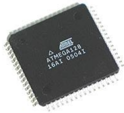
Figura 2.1.3: Microcontrolador ATmega128-16AU ( www.futurlec.com )
