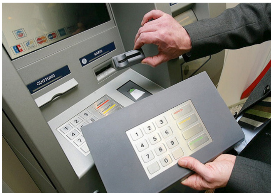
Figure 3. Old-school skimming attacks through physical means 8
