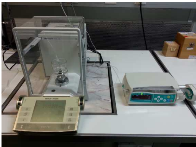
Figure 15: Calibration of a syringe pump through the gravimetric method.
