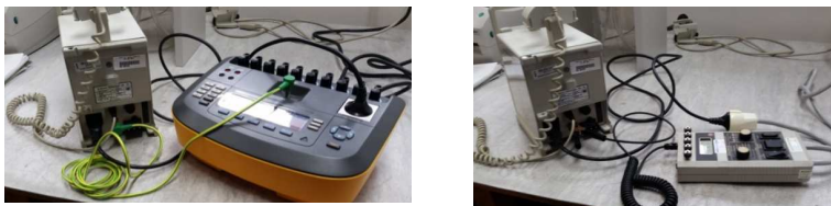
Figure 21 – Electrical security tests using a reference instrument.
