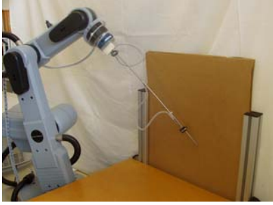
Figure 2. Steel rod impact against a rigid surface.
