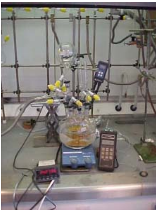
Figure 3-14. Photo of experimental set-up here. The orange colour is due to polystyrenyl lithium in methyl-cyclohexane.
