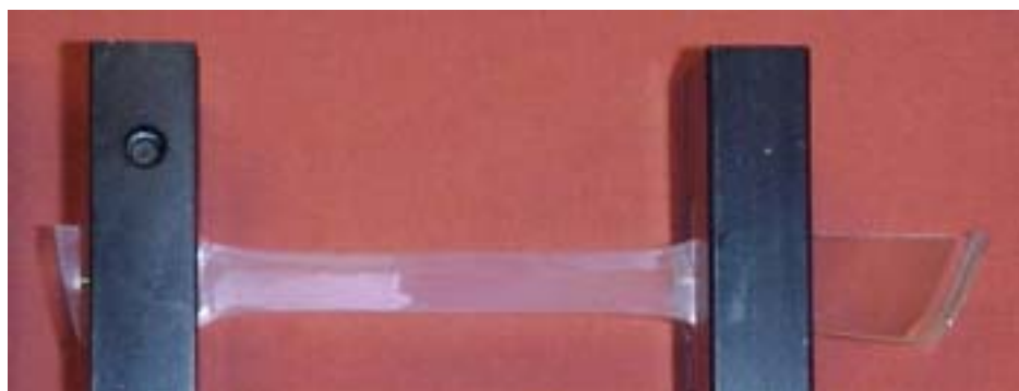
Figure 3-21. When strained the film changes from clear (outside of the clamps) to opaque (between the clamps) after a few minutes.
