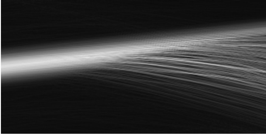
Figure 43. Example of fanning. Image of the total intensity distribution throughout the crystal. A single beam is sent through the crystal with no reflection at the end face of the crystal. The crystal is 0.25 mm wide and 1.0 mm long. The entrance surface is to the left. The c -axis points downwards.
