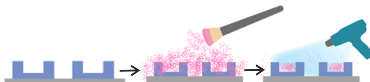
Figure 4.5: Representation of the manual loading technique for loading microcontainers. The powder is pushed into the microcontainers using a brush or a finger (middle) and the excess of powder is removed using an air gun (right).
