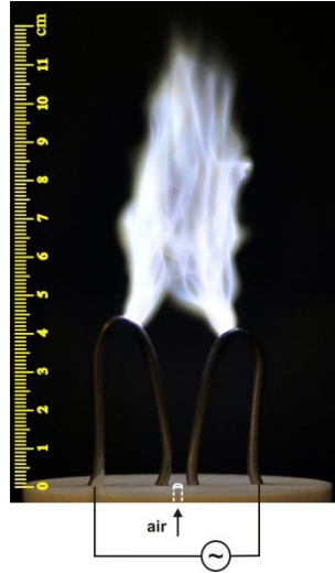
Fig. 1. Photograph of an ambient-air gliding arc discharge taken with a digital camera (Canon 350D) using an exposure time of 33 ms.
