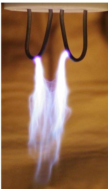
Figure 1. A photo of the gliding arc with water cooled electrodes.
