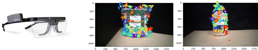
Fig. 1: Left, Tobii Pro2 Eye Tracker Glasses; Right, Fixation clustering following homography alignment
