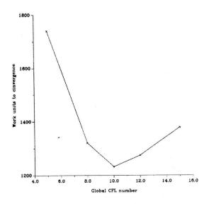
Figure 2: Comparison of the number of work units to convergence for the factored-unfactored methods with varying values of the CFL number.
