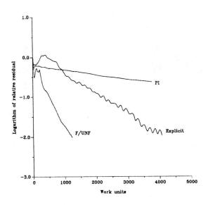
Figure 1: Comparison of convergence histories for the explicit, partially implicit (PI) and factored-unfactored (F/UNF) methods.
