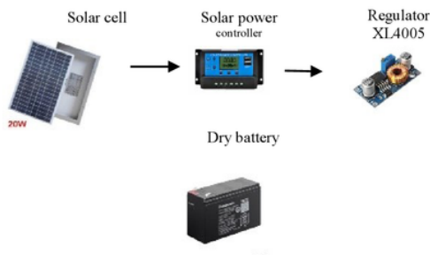
Fig. 4. Power Supply Circuits
