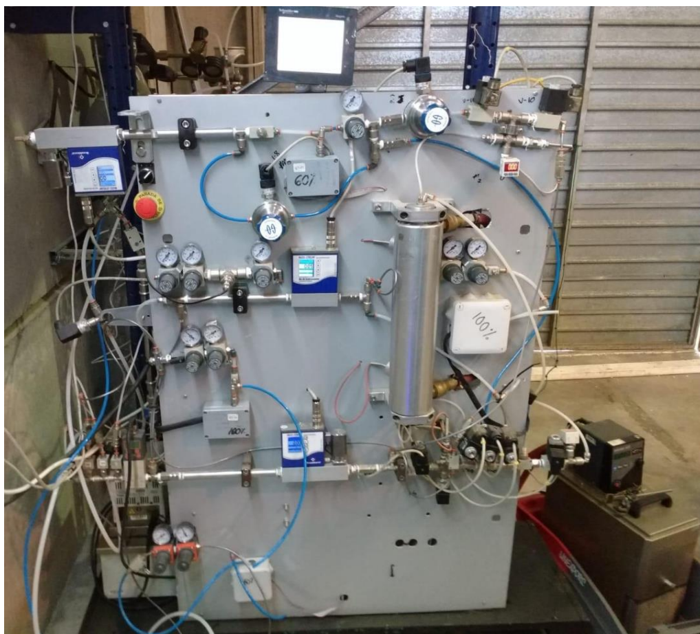
Figure 27: Picture of the single column VPSA laboratory developed.
