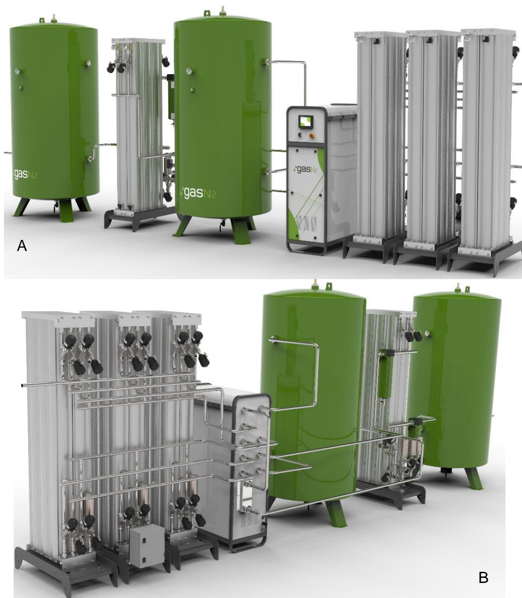
Figure 36: VPSA industrial plant design represented with a 3D model render (A) Front, (B) Back.
