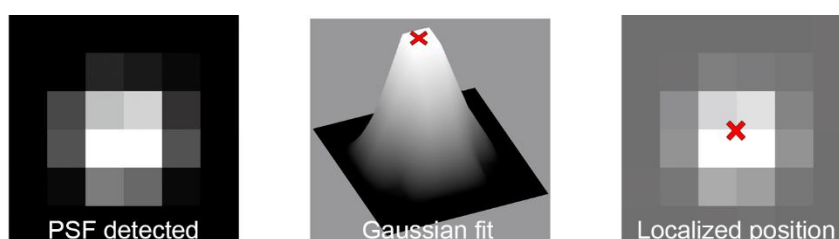
Figure 2.2 Single-molecule localization. The PSF of a single fluorophore typically shows a Gaussian shape. Fitting its intensity profile into a Gaussian distribution allows us to find the centroid (red cross), giving the localized position of the fluorophore with nanometric precision.
