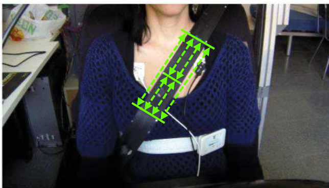
Fig. 8.3 Distances calculated between features points (dashed green arrows) to obtain the respiratory signals. The number of signals depended on the number of available feature points.
