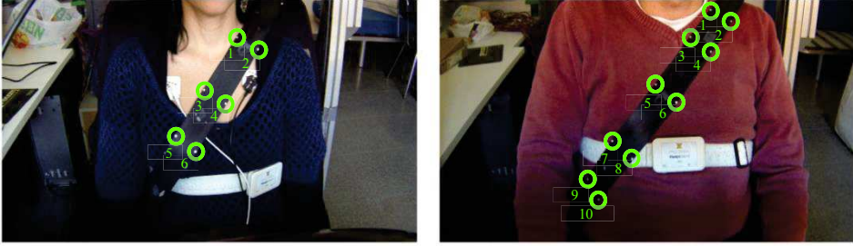
Fig. 8.1 Subjects with a different number ( n ) of reference seat belt marks (inside the green circles): (left) subject with six marks; (right) subject with ten marks. The reference marks were numbered from left to right and from top to bottom.
