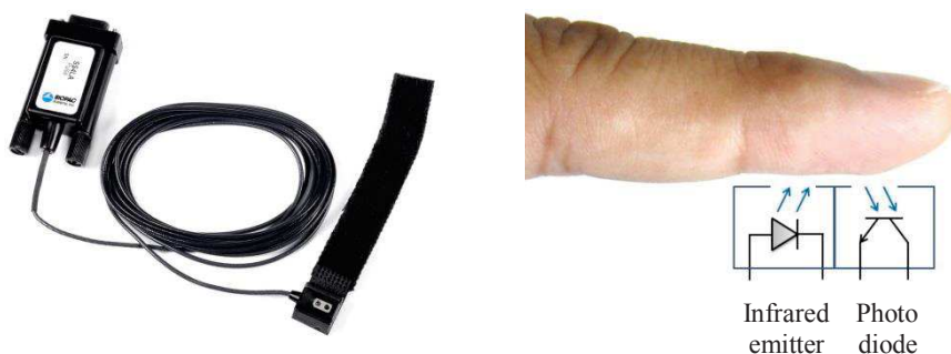
Fig. 3.4 (left) SS4LA BIOPAC Systems, Inc. finger pulse sensor; (right) diagram of the reflectance-mode PPG sensor.
