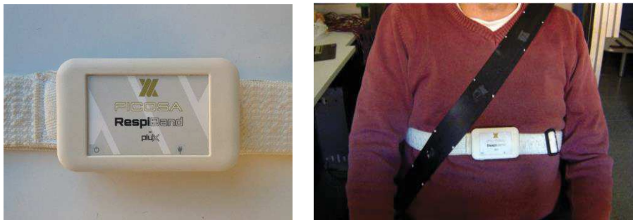
Fig. 3.9 (Left) RespiBand by plux of FICOSA International S.A.; (right) subject using the band during the recordings.
