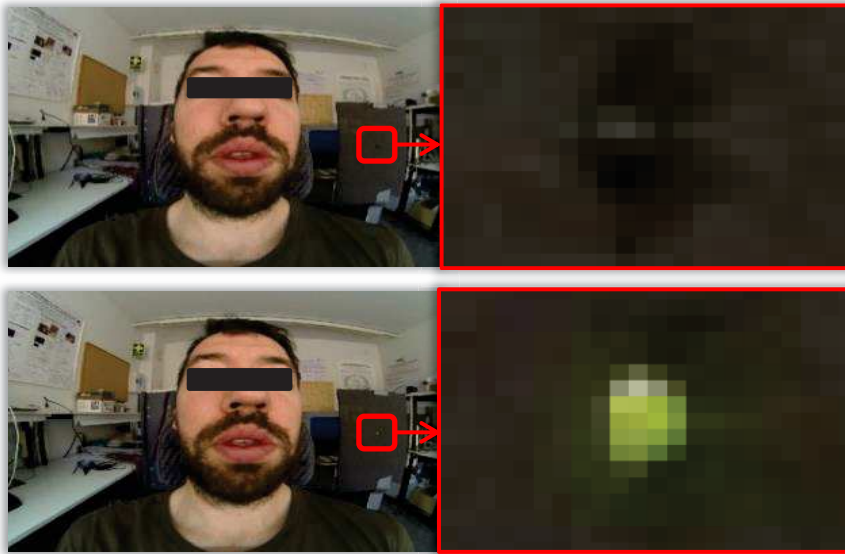
Fig. 4.8 Sawtooth signal acquisition: (top) frame with LED off; (bottom) frame with LED on.
