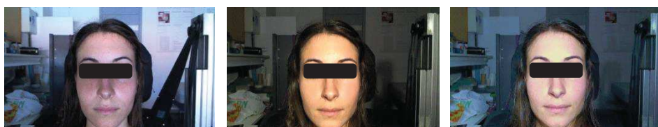
Fig. 6.1 A subject's face illuminated using different sources of illumination: (left) sunlight; (middle) LED light; (right) fluorescent light. The videos were recorded at 200 lux of illuminance with each lighting source.
