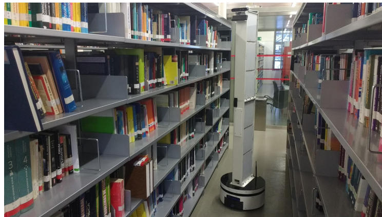
Figure 5.5: The robot at the verification setting, the University Library. Side covers removed so six RFID antennas are visible on one side.
