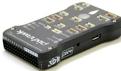
Figure 4.5: Pixhawk Autopilot, the gyroscope/accelerometer installed in the robotic subsystem. Source: https://pixhawk.org/
