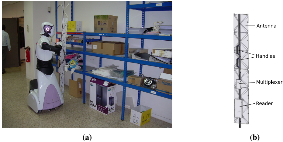
Figure 3.1: (a) Proof of concept of the mobile RFID system for inventory. Labelled objects were inside the boxes on the shelves. (b) Detail of the RFID subsystem that the humanoid robot is carrying.
