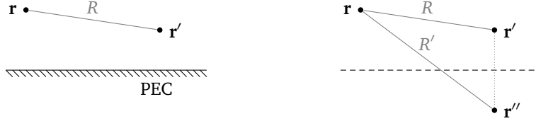
Figure 2.2: Image theory applied to the calculation of the Green's function in a half-space.
