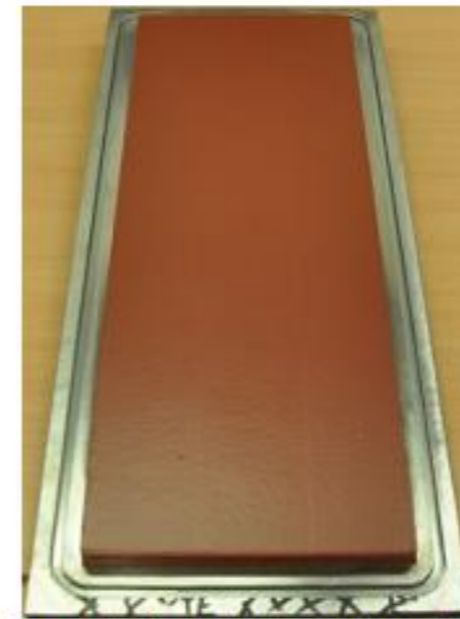
a. Coat-1 before hydrodynamic testing
