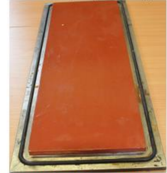
d. Coat-2 after hydrodynamic testing
