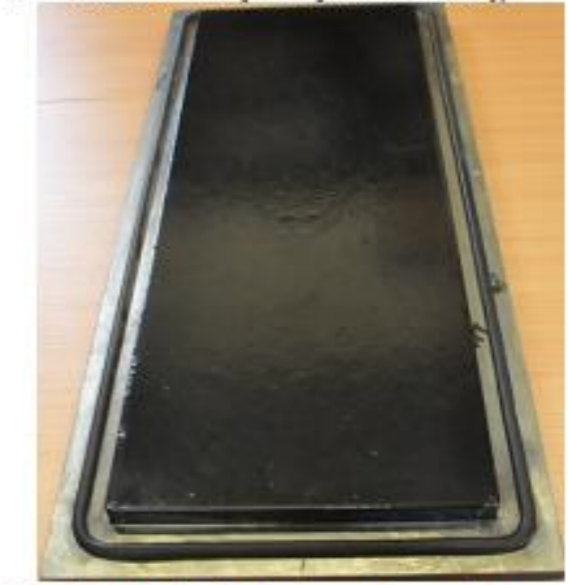
f. Coat-3 after hydrodynamic testing
