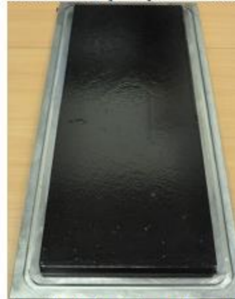
e. Coat-3 before hydrodynamic testing
