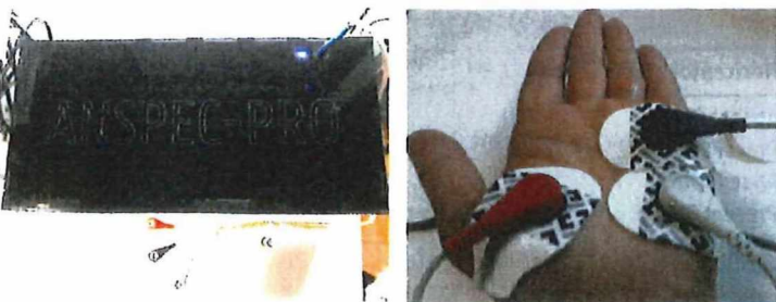
Figure 3: Left: The ANSPEC-PRO prototype for non-invasive measurement of bio-electrical skin impedance. Right: Placement of the electrodes during proof-of-concept measurements; two current carrying electrodes (white, red) and one pick-up electrode (black).
