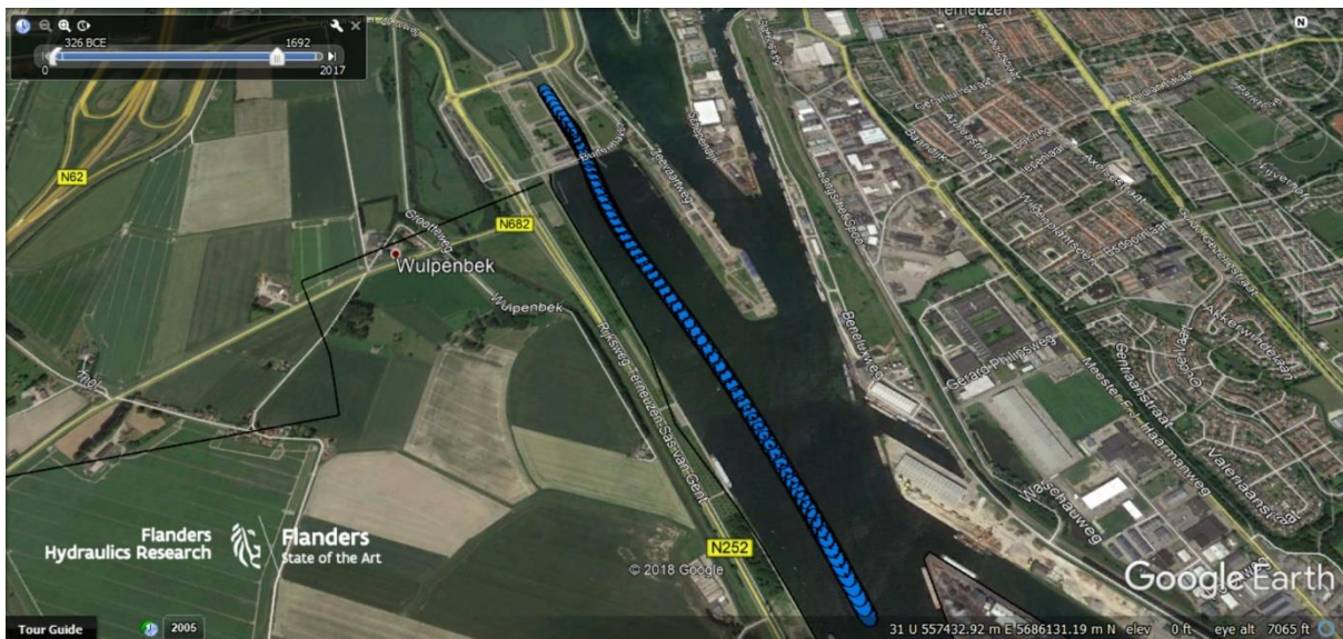
Figure 9 FT Track Controller trajectory of a 43m wide bulk carrier leaving the lock at Terneuzen sailing southbound on the Canal Gent-Terneuzen
