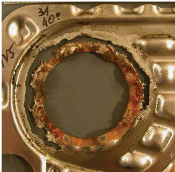
Figure 7: Crevice corrosion under the gasket of a plate heat exchanger.
