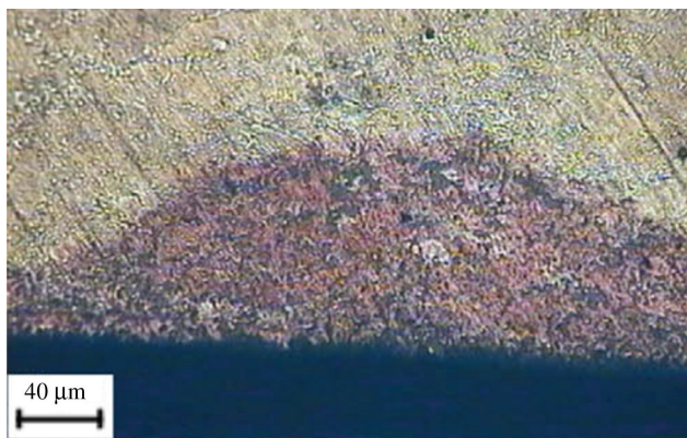
Figure 14: De-zincification of the inner surface of a yellow brass tube. Reprinted from Ranjbar (2010), with permission from Elsevier.
