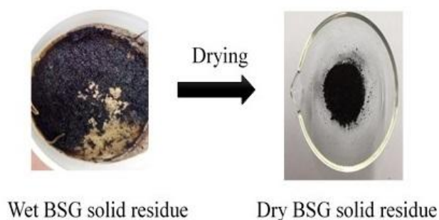
Figure 6-5: The drying process was conducted towards solid residue recovered after the liquefaction by undergone oven dry heating at 105 °C for 12 hours. The exact amount of dried BSG after the process was used for residue and conversion yield.
