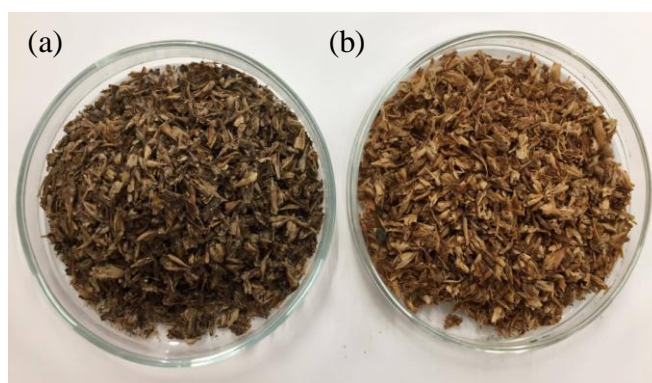
Figure 4-6: Photo of BSG (a) before extraction (b) after extraction ( extractive-free BSG ). Both samples underwent oven drying at 105°C for 24 hours.
