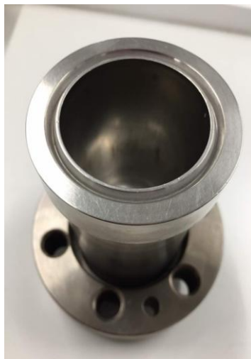
Figure 3-3: Photo of 100 mL vessel used in the autoclave reaction system for current work.
