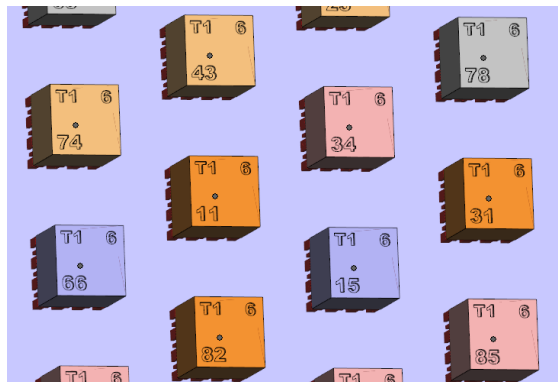
Figure 3-9: Samples labelling and arrangement on the build platform
