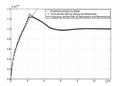
Fig. 1: Stress intensity factor (opening mode) vs. time for the Heaviside pulse
