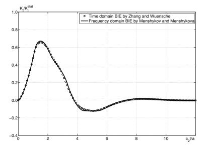
Fig. 2: Stress intensity factor (opening mode) vs. time for the triangular pulse,  $t^* = 1.12$
