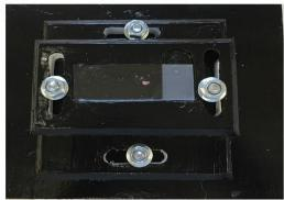
Figure 1. The handheld Raman probe in situ in the Neuropathology Department at Royal Preston Hospital. (a) Instrument setup showing (1) Raman probe, (2) sample compartment, (3) Raman detector and laser source, and (4) computer module with appropriate software. (b) A different view of the instrument setup with the sample compartment opened. (c) Sample holder with an example slide inside the sample compartment.
