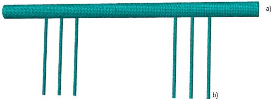
Figure 38. External Fixator mesh, constituted by a rod (a) and pins (b).
