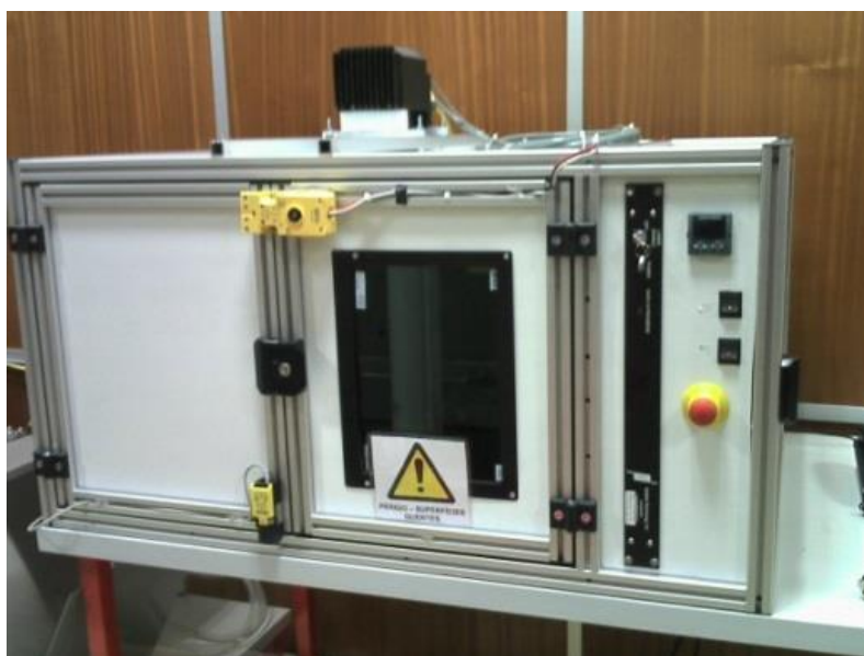
Figure 2.5 Photograph of the LaserBox equipment where the laser assisted sealing process is conducted.
