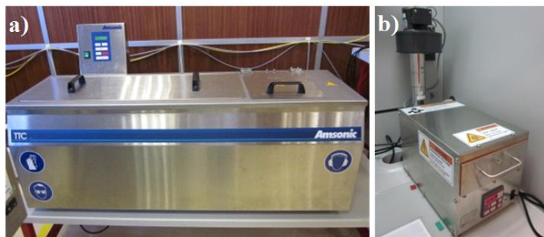
Figure 2.20 a) Ultrasounds cleaning machine (Amsonic TTC 2530) and b) UV-O 3 cleaning unit (UVO Cleaner model 42-220).
