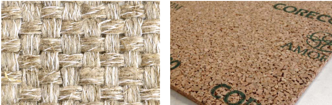
Fig. 1. Example of flax fiber configuration and cork agglomerate used.
