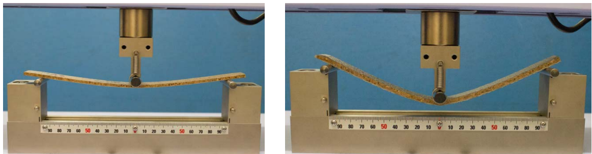
Fig. 3. Three point bending test.
