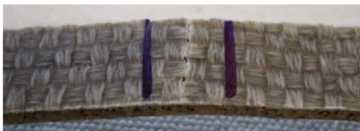
Fig. 5. Rupture on the opposite face by tensile loads.
