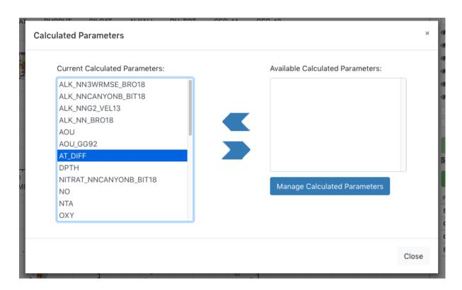
Two lists of calculated parameters appear in the screen. The list on the left are the parameters than can be used in the current layout. The list on the right are the parameters that can be added to make them available in the current project. If you need to create a parameter that is not in the list then press "Manage calculated Parameters", this other form will show up:
