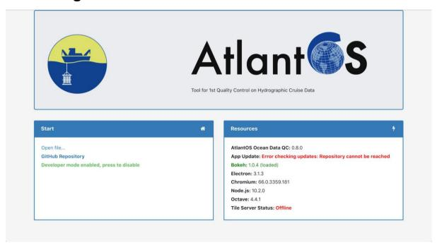
The above image is the welcome screen where there is a section informing about the actual version of the different applications and frameworks used by the application. A detection of these versions is done when launching the application and warnings will appear for notifying problems
