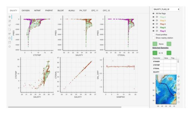
The main layout is composed by a tabbed layout of plots, defined for each parameter to do QC with, a left bar with a set of tools to interact with the plots, and a right sidebar with the information needed to do the QC, selection of parameters, visibility and flagging buttons, small table with the data for selected samples, and a bathymetric map. Detailing each section:
