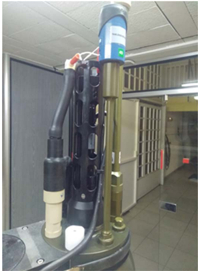
Figure 16. SeaFET pH sensor integrated on a NKE Instrumentations Provor CTS5 profiling float equipped with the OSEAN board.
