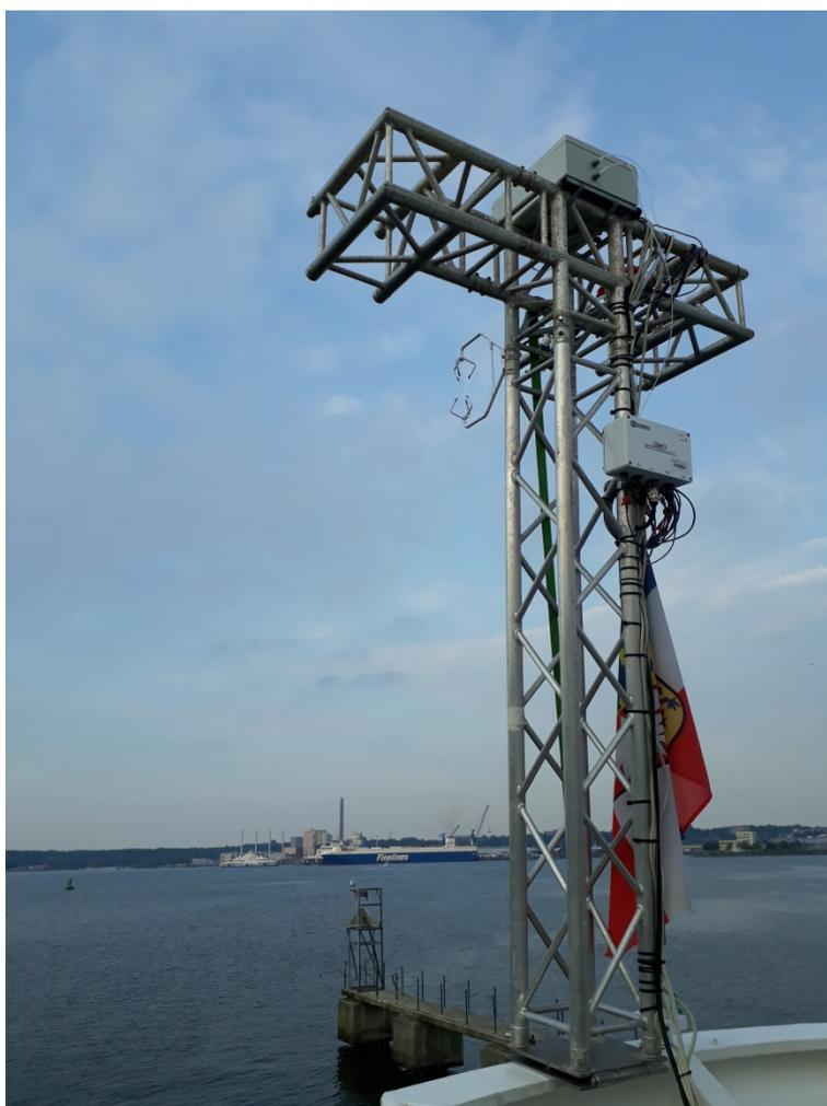
**Figure 5:** Mast including sensors and air inlet at the bow of the Alkor.
