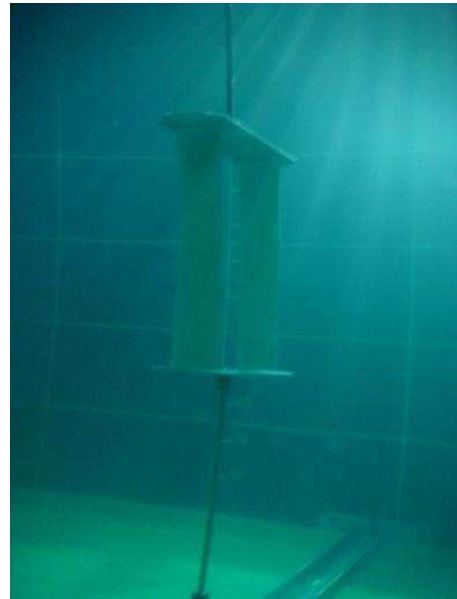
Fig. 14 Thick NACA 14 foils under test, no tail was required since the array was locked in the upper load cell.
