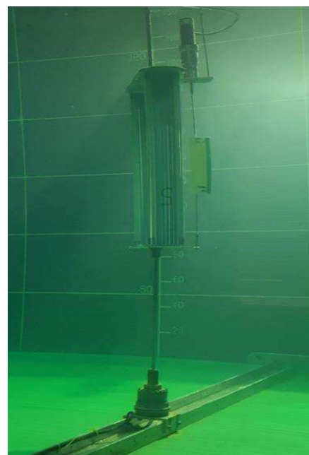
Fig. 6 The lower multi-axis load cell in situ.
