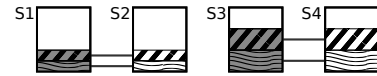
Fig. 3. Example of protection: master VNFs are running on servers S_2 and S_4 , while slave are running on S_1 and S_3 . Each link between VNF instances represents the connection between a master and its slave.
