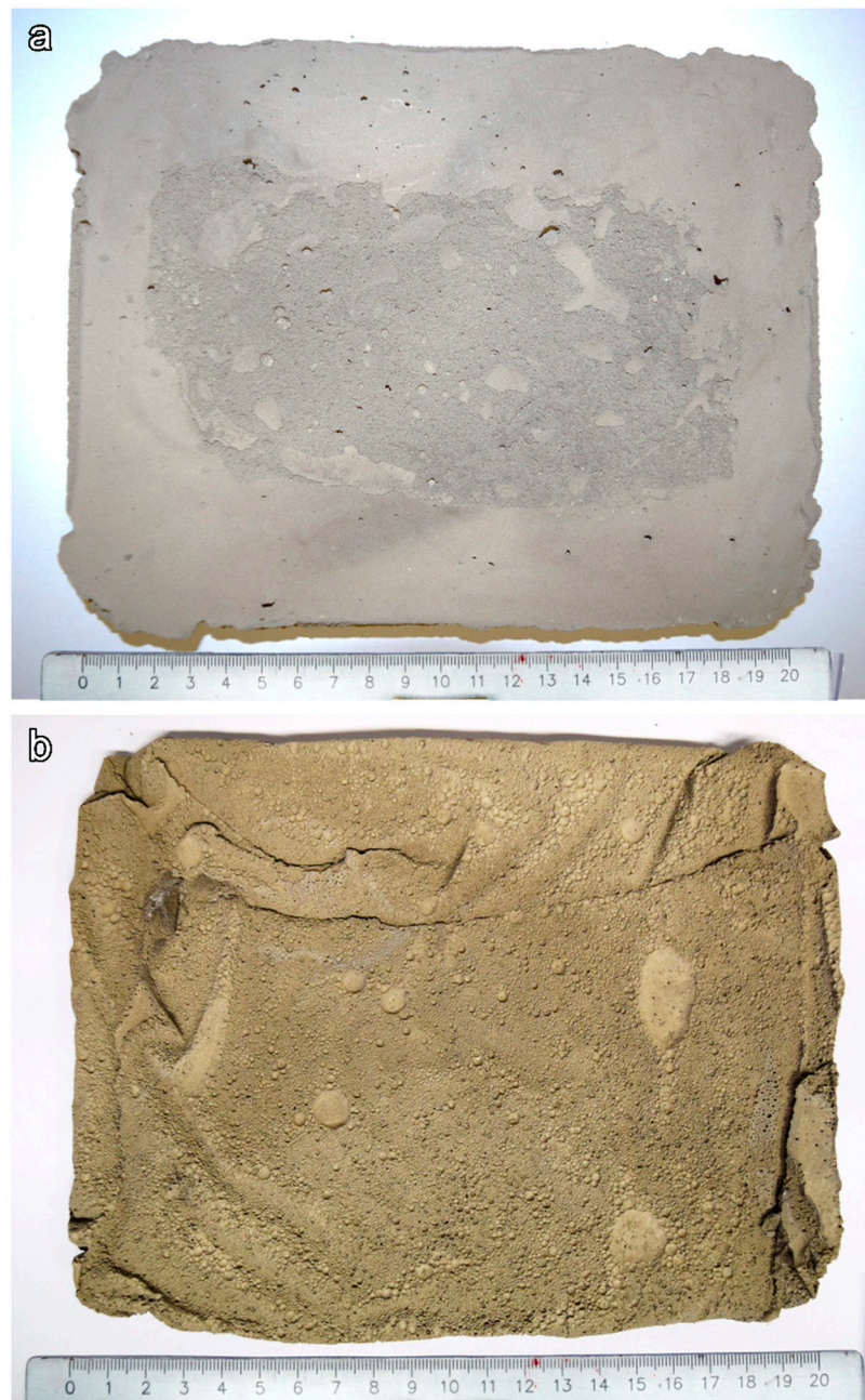
Figure 11. General view of lightweight panels; (a) 6S hardened panel; (b) heat treated panel at 800 °C.
