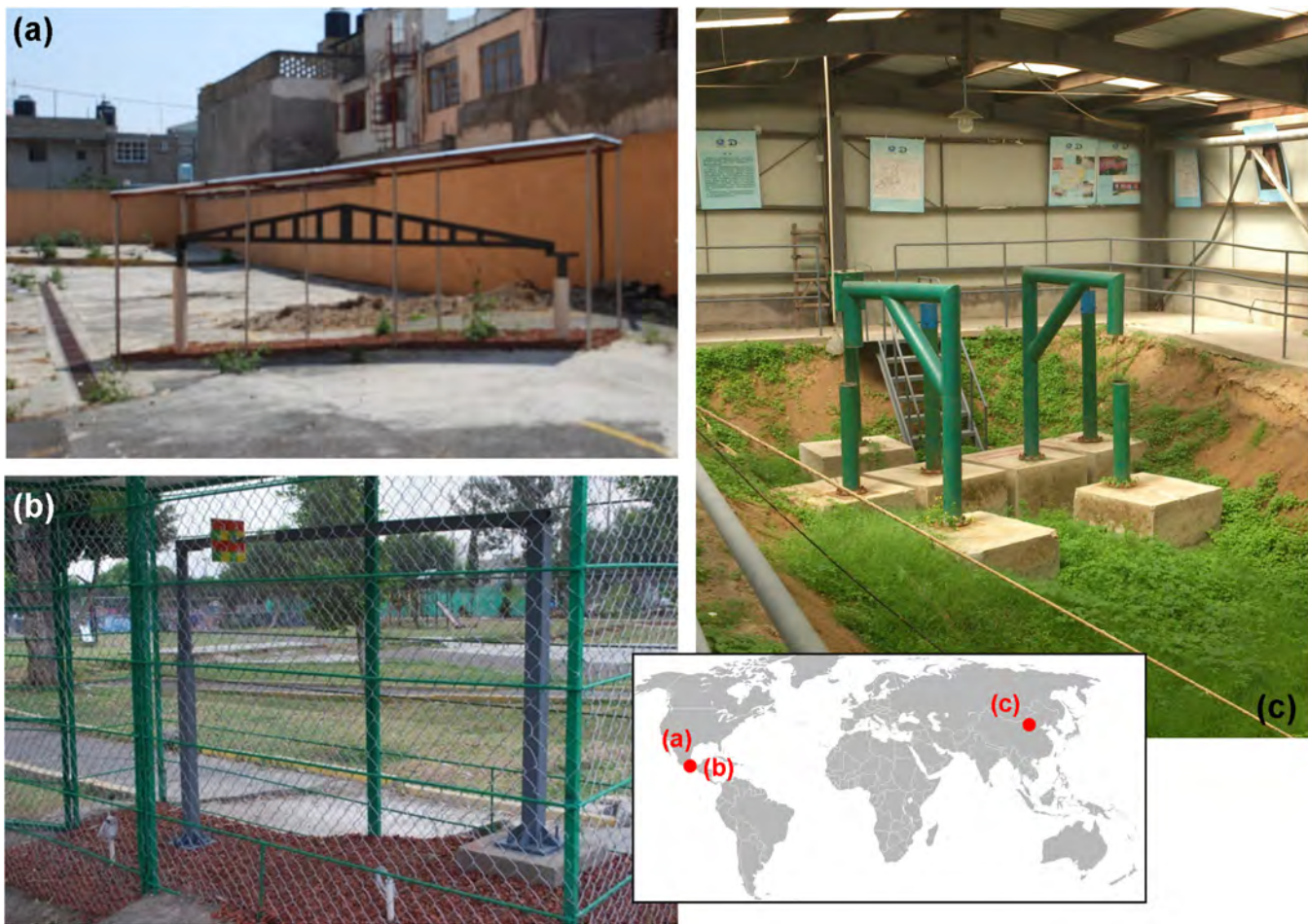
Figure 11. Some examples of ad hoc instrumentation developed to monitor opening and sliding of earth fissures or faults activated by the overdraft of aquifer resources. (a) 1-D apparatus and (b) 3-D apparatus established in Iztapalapa, Mexico City (courtesy of Dora Carreón-Freyre, Centro de Geociencias, UNAM, Mexico). (c) 3-D instrumentation installed in the northern Beijing plain (courtesy of Lin Zhu, Normal Capital University, Beijing, China).
