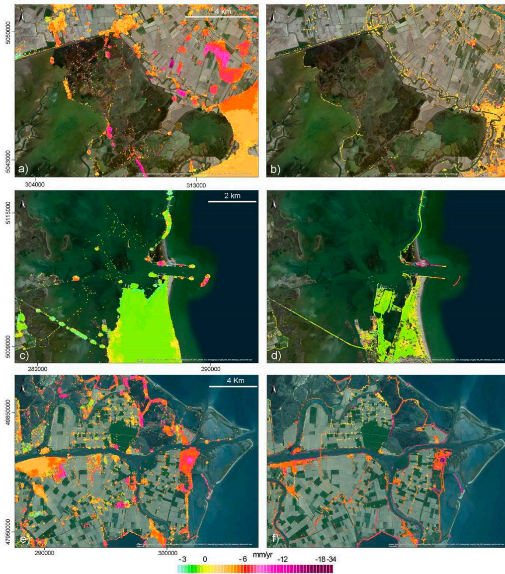
Figure 10. Average displacement rates (mm/yr) between January 2007 and July 2010 on ALOS-PALSAR images and from September 2008 to July 2011 on COSMO-SkyMed images. (a) ALOS-PALSAR outcome in the northern Venice Lagoon; (b) COSMO-SkyMed outcome in the northern Venice Lagoon; (c) ALOS-PALSAR outcome in the southern Venice Lagoon; (d) COSMO-SkyMed outcome in the southern Venice Lagoon; (e) ALOS-PALSAR outcome in the Po River Delta; (f) COSMO-SkyMed outcome in the Po River Delta. Negative values indicate subsidence, positive mean uplift. The image background is from Esri, DigitalGlobe, GeoEye, Earthstar Geographics, CNES/Airbus DS, USDA, USGS, AEX, Getmapping, Aerogrid, IGN, IGP, Swisstopo, and the GIS User Community.
